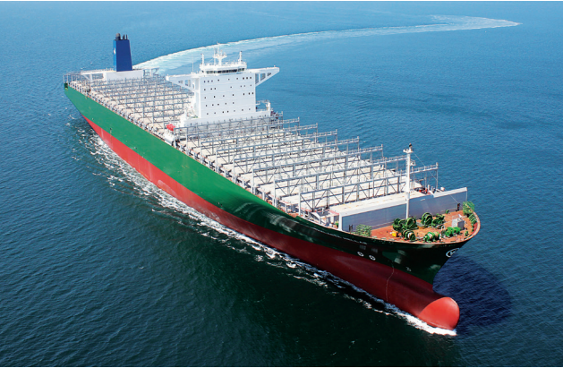
Thalassa Hellas containership delivered In September 2013, we delivered this 13,800 TEU containership to Enesel of Greece, the first of ten vessels ordered in 2012. In addition to optimized fuel efficiency thanks to an improved hull form, main engine low-load tuning with exhaust gas boiler, and other energy-saving features, the vessel is equipped with our Hi-Ballast ballast water treatment system, helping it earn the GL Environmental Passport notation.
