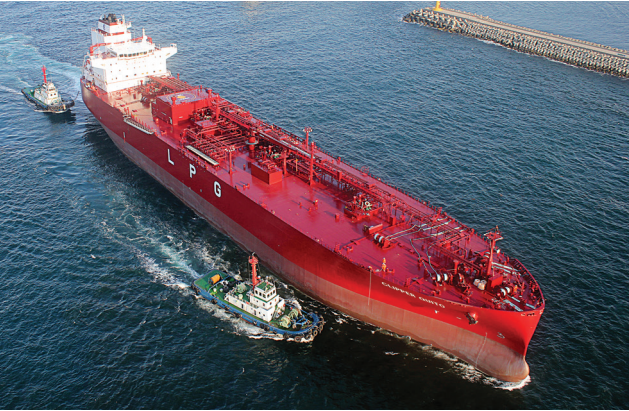
Clipper Quito LPG carrier delivered In June 2013, we delivered this 84,000 cbm LPG carrier to Solvang ASA of Norway. In addition to an improved hull form that maximizes fuel efficiency, the vessel is equipped with an advanced exhaust gas cleaning system that enables it to meet new IMO emissions regulations while running on low-cost heavy fuel oil rather than high-cost low-sulfur fuels such as marine gas oil.
