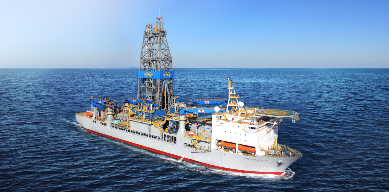
Noble Don Taylor drillship delivered In April 2013, we delivered this deepwater drillship to Noble Drilling of the US. Capable of drilling at depths of up to 12,000 ft, this purpose-designed vessel is optimized to improve fuel efficiency as well as for improved position-holding during drilling operations. The thruster canisters allow maintenance and repairs to be carried out in the field, saving both time and money.
