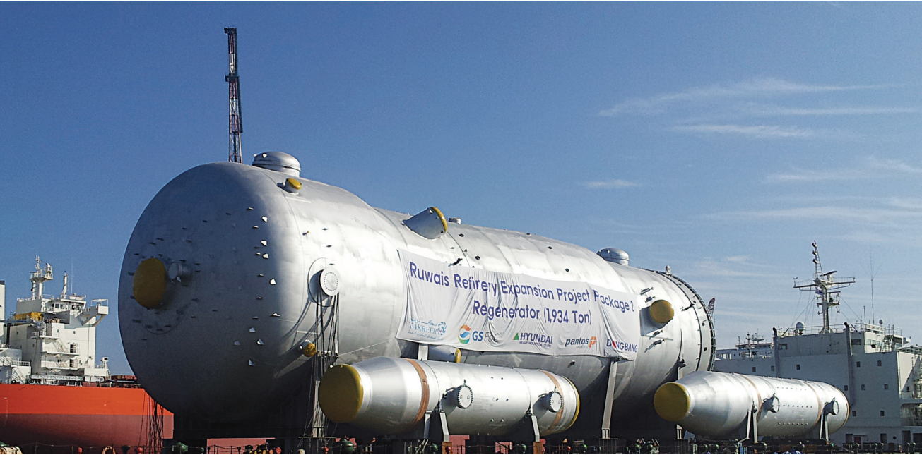
Ruwais Refinery RFCC Project In August 2011, we delivered this regenerator to GS Engineering & Construction for the Ruwais Refinery Expansion Project in the UAE. At 60-meters tall, 16-meters in diameter, and 1,934 tons in weight, the unit is the largest of its kind to date.
